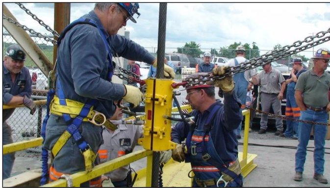
Alliance Coal, Indiana, USA. Dynagard LVL being applied with JU16L System
